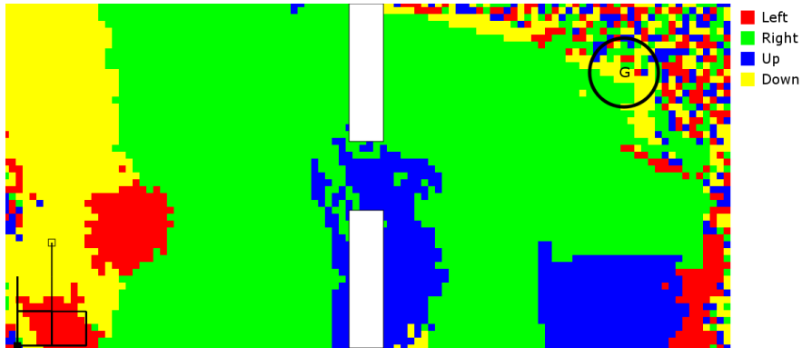
Figure 2.8: Example policy during the second run of an experiment in the 2D environment. The colors depict the action the agent reckons most valuable in each state (see legend). The goal area is designated by a circle and 'G'. The trajectory of the second run is overlaid on the policy with a black line. The trajectory's start state is designated with an open square. The agent's policy forces him into the lower left corner, where he gets stuck.
