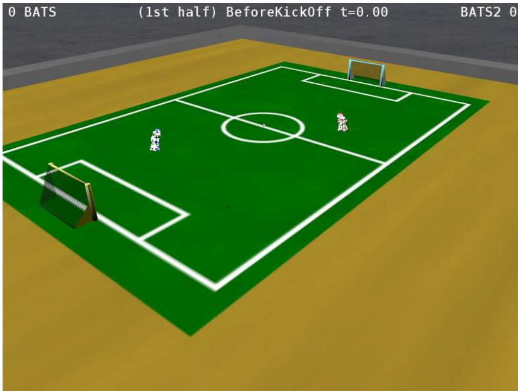
Figure 1.1: The 3D Football simulation field. The field is 12x8 meters in size and contains two colored goals and the ball. Two humanoid agents are placed in the field. At the top of the simulator window the scores, game state and game time are shown.
