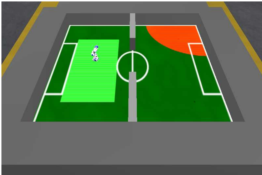
Figure 2.2: 3D simulation field used in RL experiment. The light green area denotes the starting area, the red circle the goal area. This environment is also divided in two parts by placing obstacles. Compare to figure 2.1
