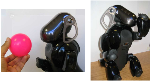
Fig. 2. Sony Aibo ERS-7, Left: with pink ball, Right: hiding head while playing "peekaboo". The camera vision is partially obscured by the arm.
