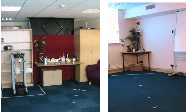
Fig. 5: Views of simulated living room showing robot and the 0.5m scale marked diagonally on the floor
