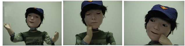
Fig. 2. End postures of three dynamic expressions of KASPAR used in the current work (including facial expressions and gestures).
