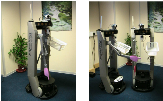
Fig. 1: The PeopleBot™ robots fitted with a pointer (in raised and lowered positions) and basket.
