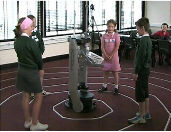
Fig. 3: A child being selected by the robot while playing the Rotation Game, with pointer rising to point to him (active pointer mode). Spatial zones are marked on floor.
