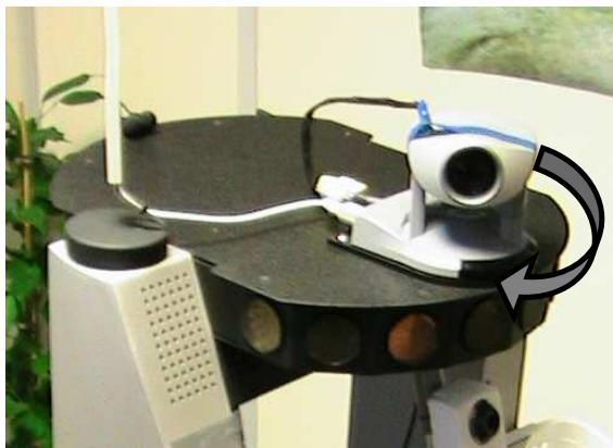
Fig. 2: Extent of the robot's camera movement
