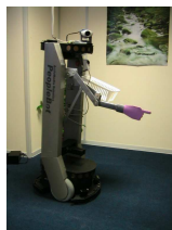
Fig. 1 PeopleBot™ robot with the lifting arm used in the children's robot trials
